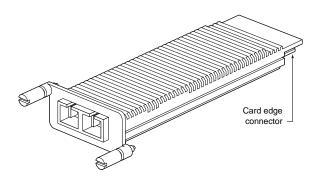
Figure 19: XENPAK Module
